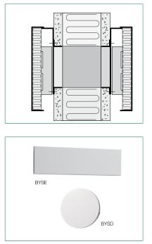
Transfer air device BYSE, BYSO is intended for positioning on a wall, and can be used in most environments. The devices provide good sound attenuation and are easy to install. They are made from hot-dip galvanized steel sheet. Visible parts are powder-coated for a high surface finish and good impact and scratch resistance.
